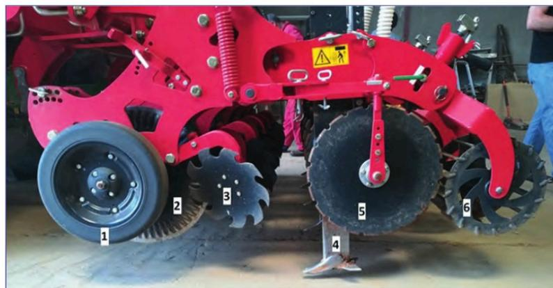
**Figura 5** Tren de laboreo en bandas del Farnet Strip-Till.
